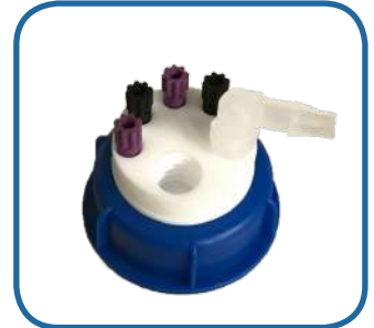
SWB-4-C-1L : 4 entries 1/8", 1 threaded barbed fitting and charcoal cartridge emplacement
